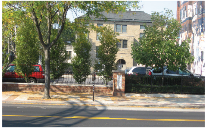
Surface parking lots should be screened from the public sidewalk by extensive landscaping and other architectural features like brick retaining walls and ornamental fences.
