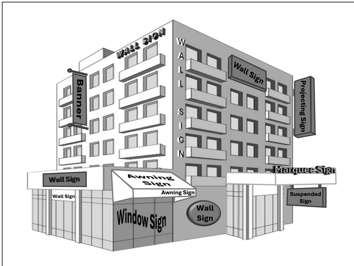
Figure C. Permanent building sign types include window signs and projecting signs. Note that not all building sign types are represented.
