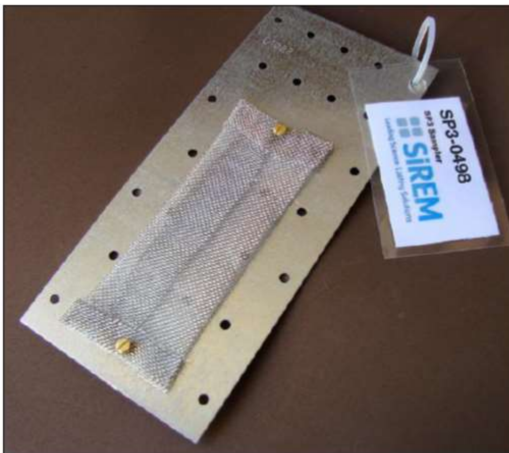
Figure 3. Low Density Polyethylene Passive Sampler
