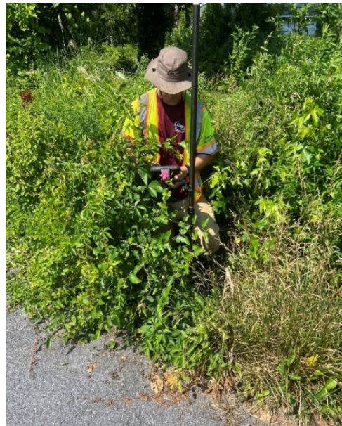
Photo 6 – Surveying outfall invert and nearby marsh elevations
