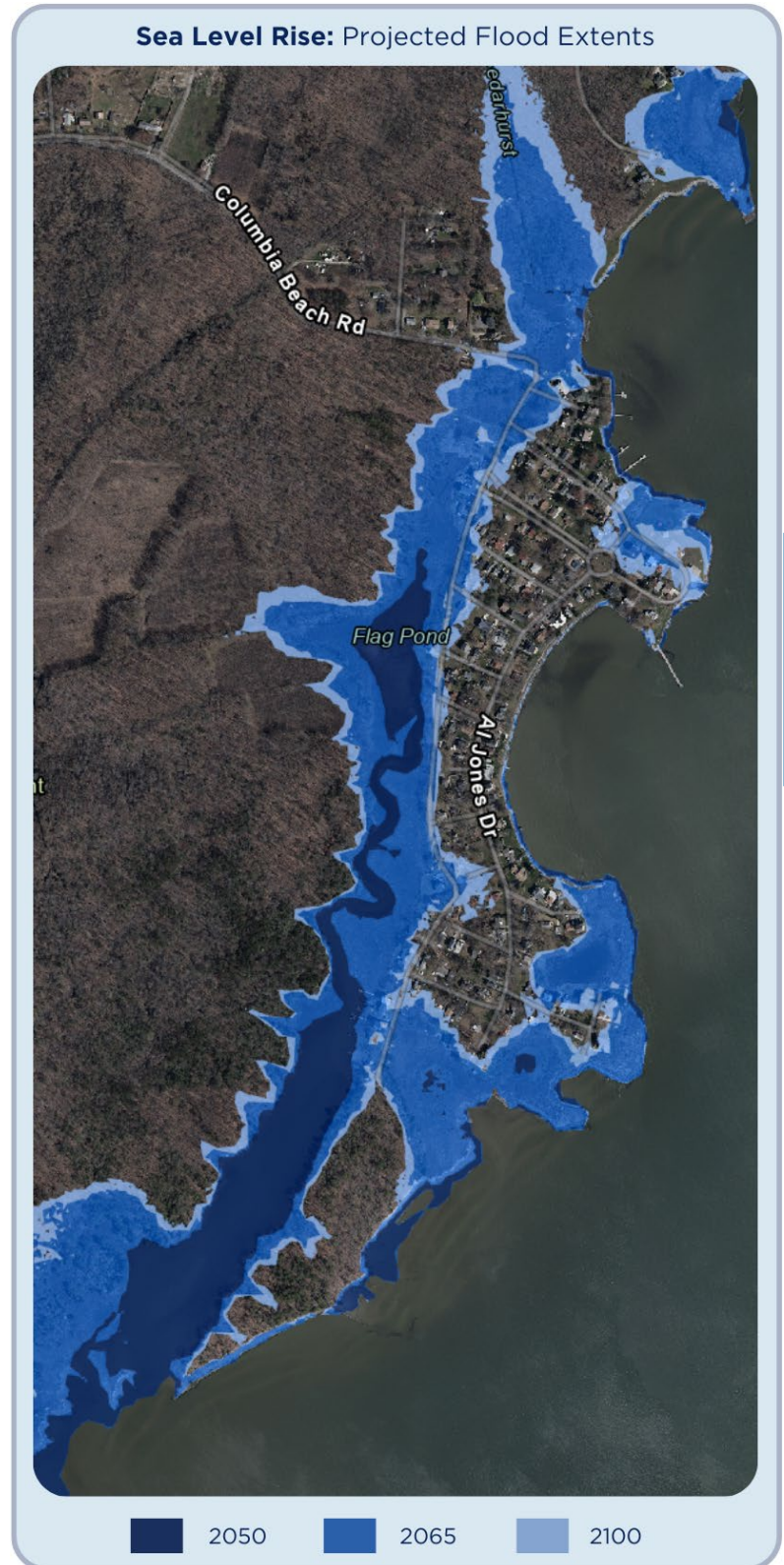
Figure 34 – Projected SLR Impacts for Columbia Beach, illustrating increasing inundation from the Chesapeake Bay and the surrounding marsh.
