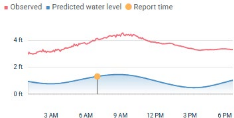
Figure 58 – Maryland MyCoast Report Documenting Property Flooding along Rockhold Creek Shoreline in Owings Beach during Tropical Depression Debby (August, 9, 2024) Water level: +4.1’ NAVD88 (or 3.44’ above MHW)
