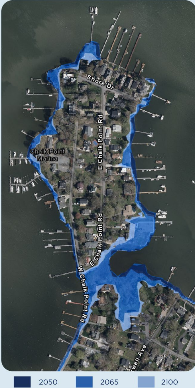
Figure 36 – Projected SLR Impact on Chalk Point Road, illustrating increasing inundation risks, particularly along the community's only access road.
