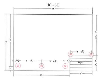
2×10 LEDGER BOARD FLASHED AND BOLTED TO HOUSE RIM WITH
