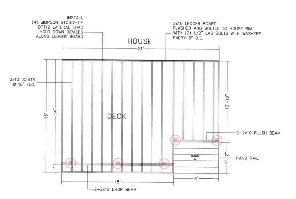
2×10 LEDGER BOARD FLASHED AND BOLTED TO HOUSE RIM WITH (2) 1/2" LAG BOLTS WITH WASHERS EVERY 8" O.C. JOISTS TO BE 2x12 SYP TREATED INSTALLED 16" O.C. BEAMS TO BE 2-2x12 SYP TREATED NAILED SUPPORT POSTS TO BE 6x6 TREATED DECKING TO BE 5/4 x 6 TIMBERTECH WESTBURY RAILS TO BE 36" HIGH WITH LESS THAN 4" OPENINGS PER IRC CODE ALL DECK HARDWARE TO BE CORROSION RESISTANT AND INSTALLED PER MANUFACTURERS INSTRUCTIONS STAIRS TO BE BUILT MAX 7-3/4" RISE 10" MIN RUN PER IRC CODE
