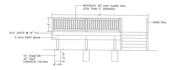
2x10 LEDGER BOARD FLASHED AND BOLTED TO HOUSE RIM WITH
