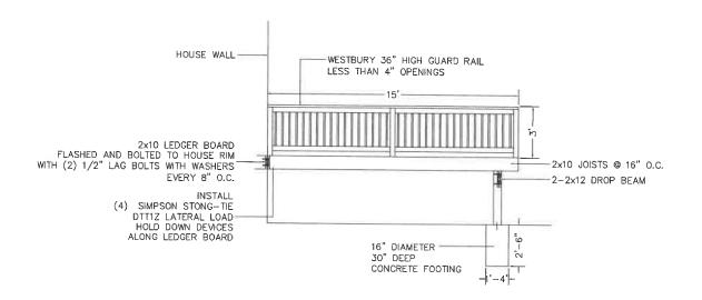
2x10 LEDGER BOARD FLASHED AND BOLTED TO HOUSE RIM WITH (2) 1/2" LAG BOLTS WITH WASHERS EVERY B" O.C. JOISTS TO BE 2x12 SYP TREATED INSTALLED 16" O.C. BEAMS TO BE 2-2x12 SYP TREATED NAILED SUPPORT POSTS TO BE 6x6 TREATED DECKING TO BE 5/4 x 6 TIMBERTECH WESTBURY RAILS TO BE 36" HIGH WITH LESS THAN 4" OPENINGS PER IRC CODE ALL DECK HARDWARE TO BE CORROSION RESISTANT AND INSTALLED PER MANUFACTURERS INSTRUCTIONS STAIRS TO BE BUILT MAX 7-3/4" RISE 10" MIN RUN PER IRC CODE
