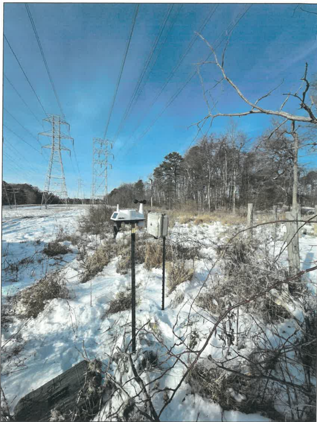
Figure D-12 Location 3 Ambient Survey Sound Level Meter & Weather Station
