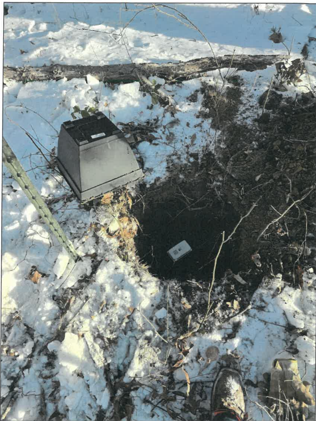
Figure D-13 Ambient Survey Vibration Meter Deployment - Typical
