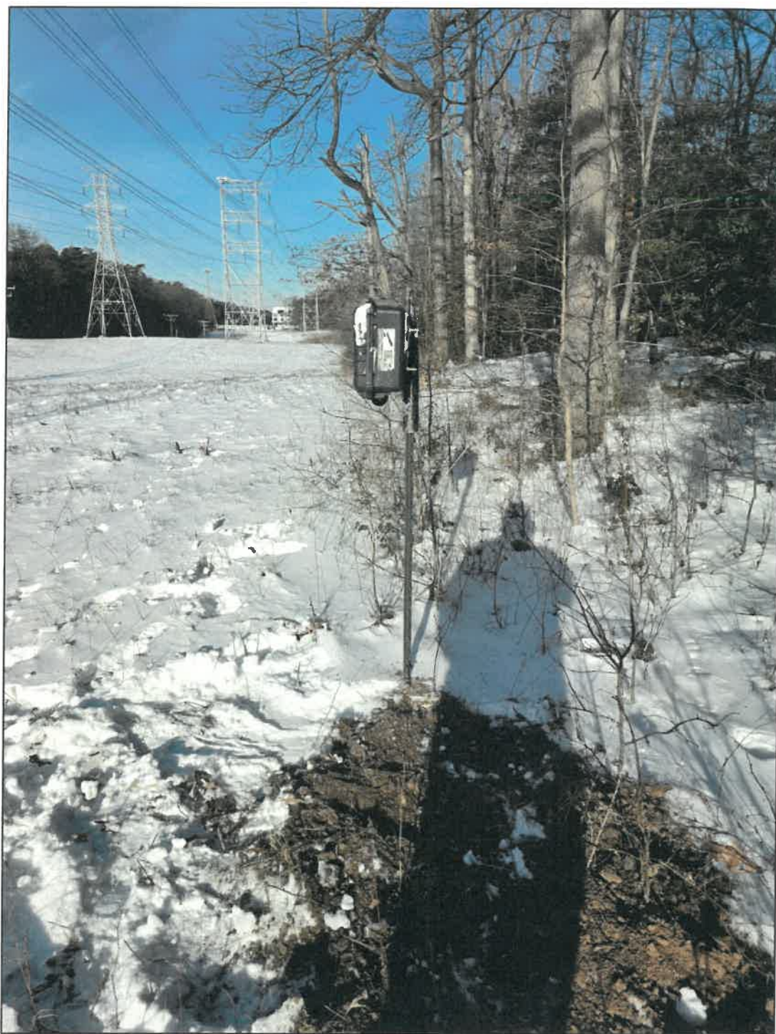
Figure D-7 Location 2 Ambient Survey Sound Level Meter
