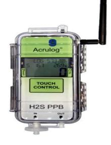
Higher sensitivity monitors placed along the plant fence line and in the community measure H<sub>2</sub>S in Parts Per Billion (ppb)
