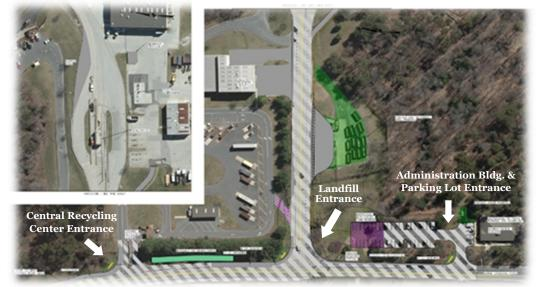
The anticipated entrance improvements include upgrades to lane widths, pavement, signage, markings, lighting, and landscaping. The County is also upgrading the parking lot adjacent to the Administration Building to enhance pavement condition and provide fully compliant accessible parking.
