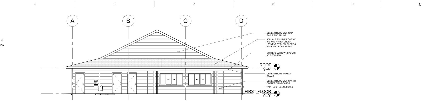
GUTTERS W/ DOWNSPOUTS AS REQUIRED. \_ROOF 9'-4" CEMENTITIOUS TRIM AT BEAMS CEMENTITIOUS SIDING WITH CORNER TRIMBOARDS PAINTED STEEL COLUMNS FIRST\_FLOOR 0'-0" A
