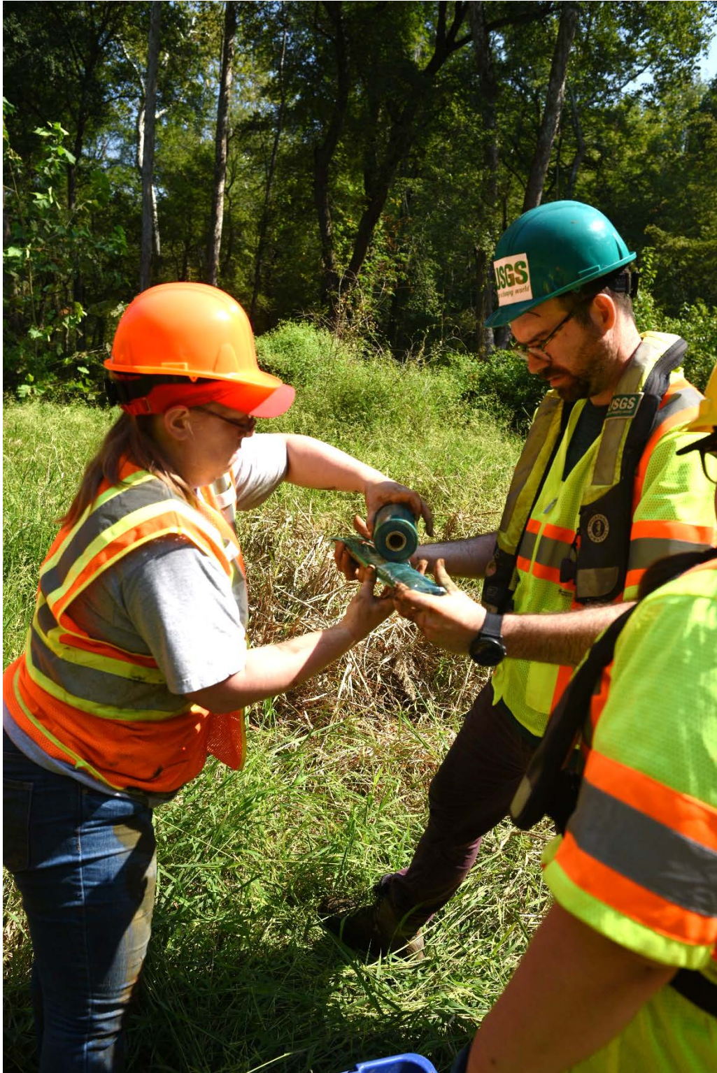
Figure 8: USGS scientists carefully wrap Russian peat core segment from the sedge clearing (most downstream sample point) in Bacon Ridge Branch near Chesterfield Road in Annapolis.
