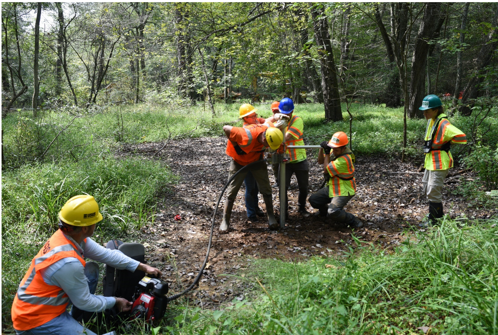
Figure 3: USGS scientists insert a vibracore sample in a floodplain depression at Bacon Ridge Branch near Chesterfield Road in Annapolis.
