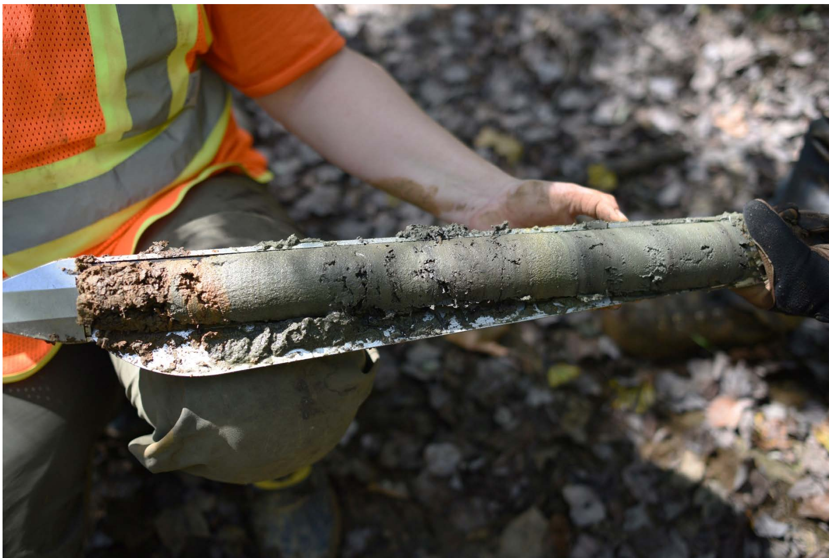
Figure 5: Distinct fine and sand layers are visible in the first segment (0-50 cm) of a Russian peat core sample collected in a floodplain depression at Bacon Ridge Branch near Chesterfield Road in Annapolis.
