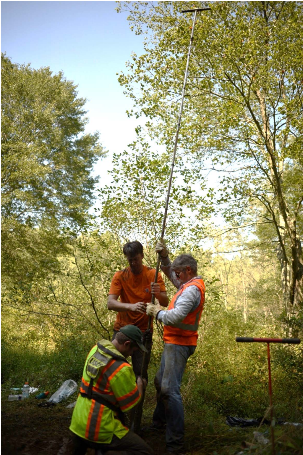
Figure 14: USGS scientists retrieve length of Russian peat corer at the sample location in marshy conditions upstream of Chesterfield Road in Bacon Ridge Branch in Annapolis. Full length of core was approximately 4.8 meters of high-quality uncompacted sediment.
