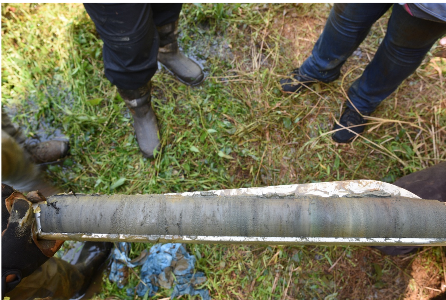
Figure 15: Clear bands of fine sediment are exposed within a Russian peat corer segment at the sample location in marshy conditions upstream of Chesterfield Road in Bacon Ridge Branch in Annapolis. Full length of core was approximately 4.8 meters of high-quality uncompacted sediment.
