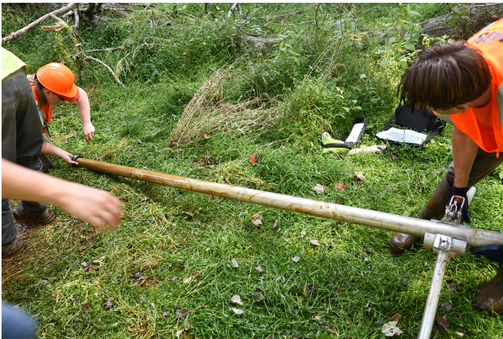
Figure 2: USGS scientists cap a vibracore sample in the floodplain at Bacon Ridge Branch near Chesterfield Road in Annapolis.
