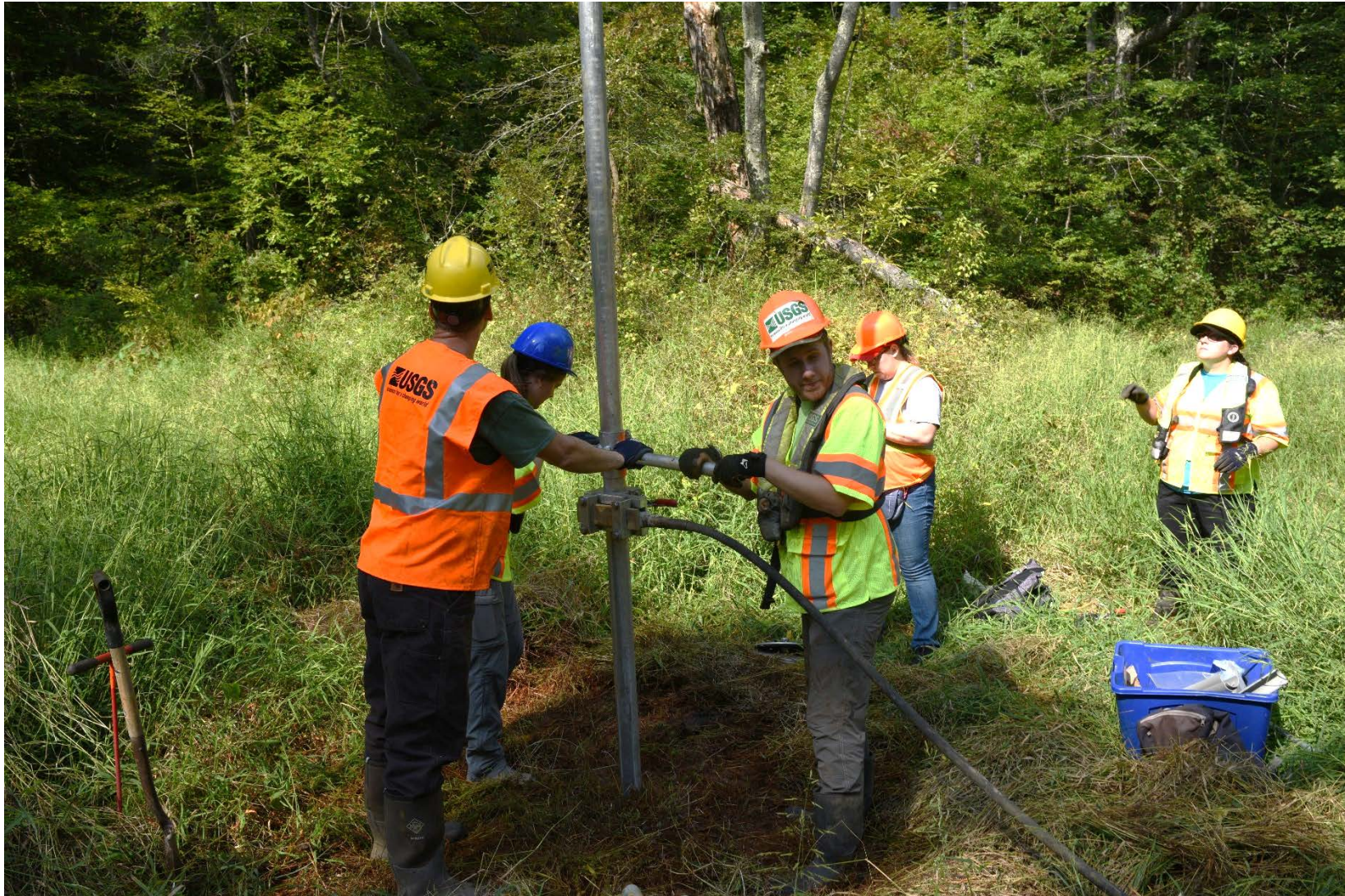
Figure 6: USGS scientists await the signal to begin vibracore collection in a sedge clearing (most downstream sample point) in Bacon Ridge Branch near Chesterfield Road in Annapolis.
