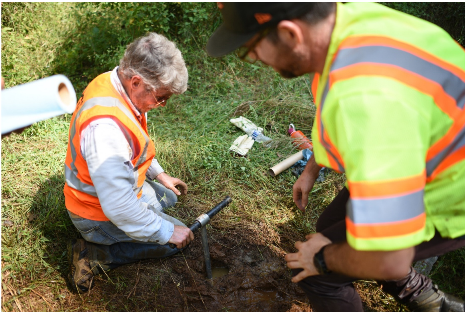
Figure 13: USGS scientists complete collection of Russian peat corer segment 7 of at the sample location in marshy conditions upstream of Chesterfield Road in Bacon Ridge Branch in Annapolis.
