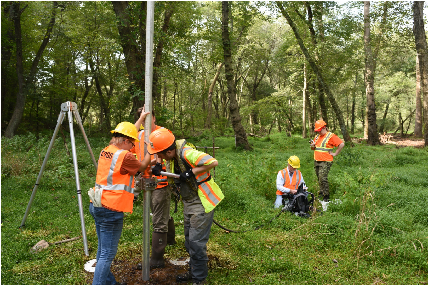
Figure 1: USGS scientists begin vibracore sampling in the floodplain at Bacon Ridge Branch near Chesterfield Road in Annapolis.
