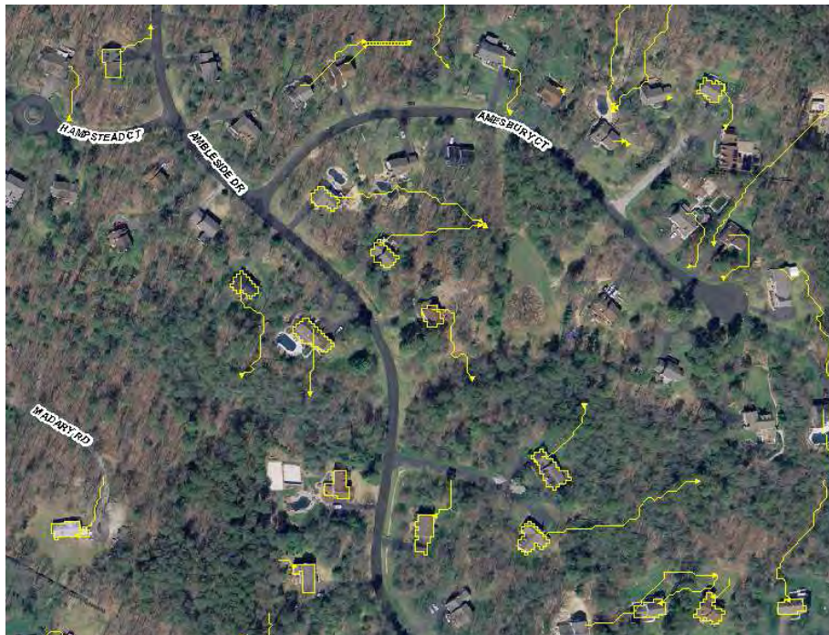
Exhibit 3: Disconnected Rooftops and Their Pervious Flow Path
