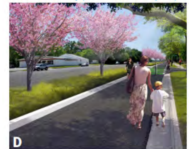
Figure 27: A Shared-use path may be used on any street. More protection becomes increasingly necessary with higher travel lanes, traffic speeds, and traffic volumes.
