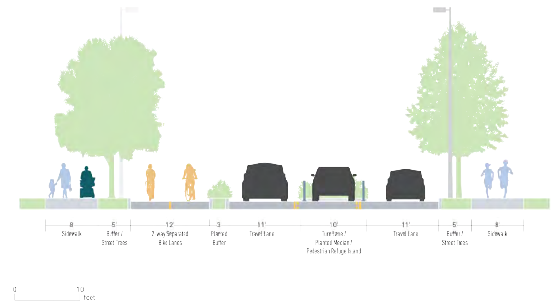
Figure 49: Recommended cross section for a street with a bi-directional separated cycle track.
