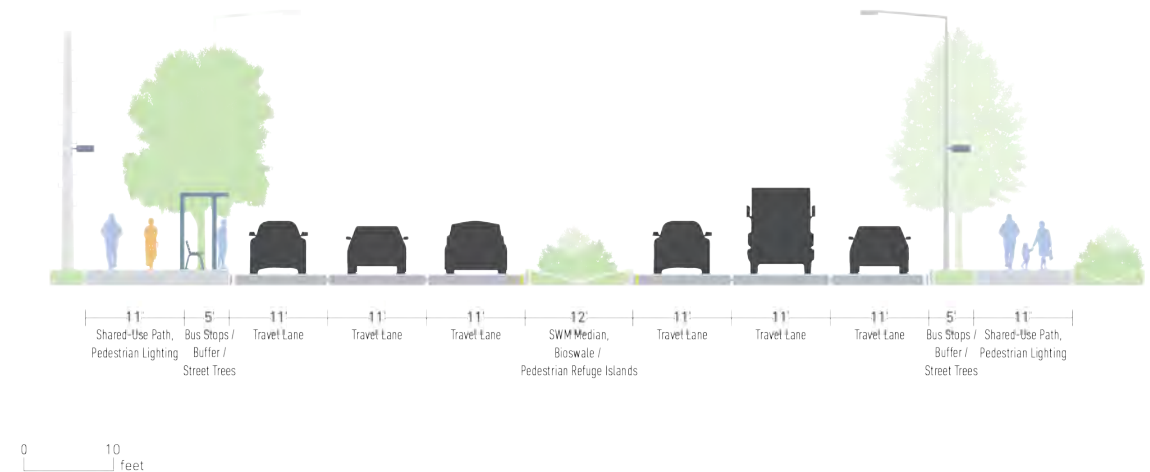
Figure 45: Recommended street design on Commercial Corridor Arterials with three travel lanes in each direction.
