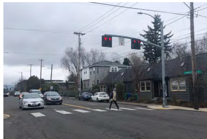
Figure 28: A Pedestrian Hybrid Beacon. Picture taken by Toole Design Staff.
