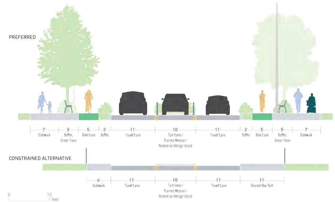
Figure 43: Recommended street design, and alternative street design in constrained areas, on Suburban Collectors.
