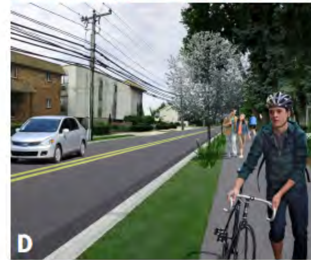
Figure 27: A Shared-use path may be used on any street. More protection becomes increasingly necessary with higher travel lanes, traffic speeds, and traffic volumes.
