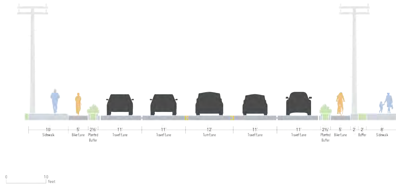
Figure 51: Recommended cross section for commercial suburban arterials.
