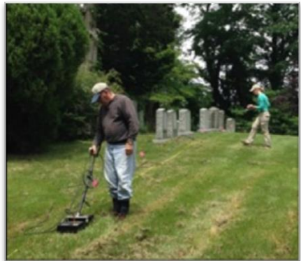
A Ground Penetrating Radar survey underway at Whitehall Cemetery.
