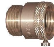
These are one of the least expensive and most commonly used backflow preventers. When attached to an outside water tap, these backflow preventers keep water that may be contaminated from entering your drinking water. If you have a sprayer on your hose you should
