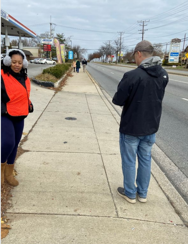
Figure 15 Frequent driveways increase the number of conflict points between drivers, pedestrians, and bicyclists. The width increases the length of exposure for pedestrians and bikes.
