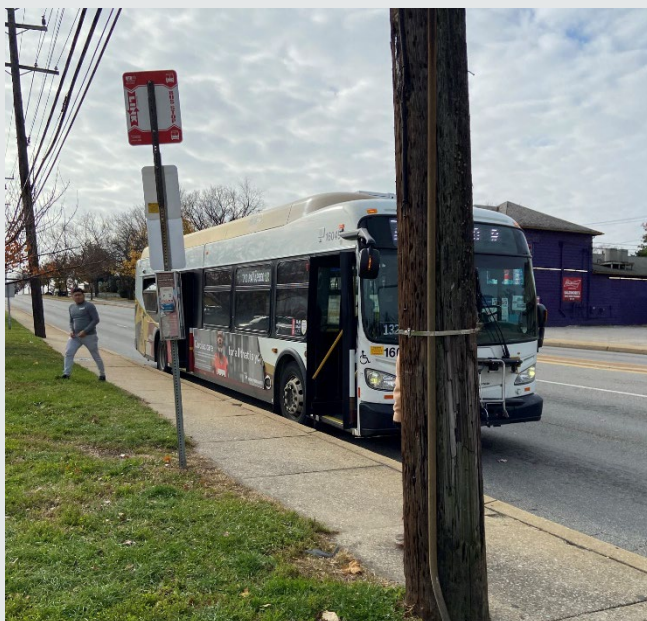
Figure 14 Many bus stops do not have a shelter, seating or properly sized pad. Many people take shortcuts away from the narrow sidewalks on Ritchie Highway as shown.
