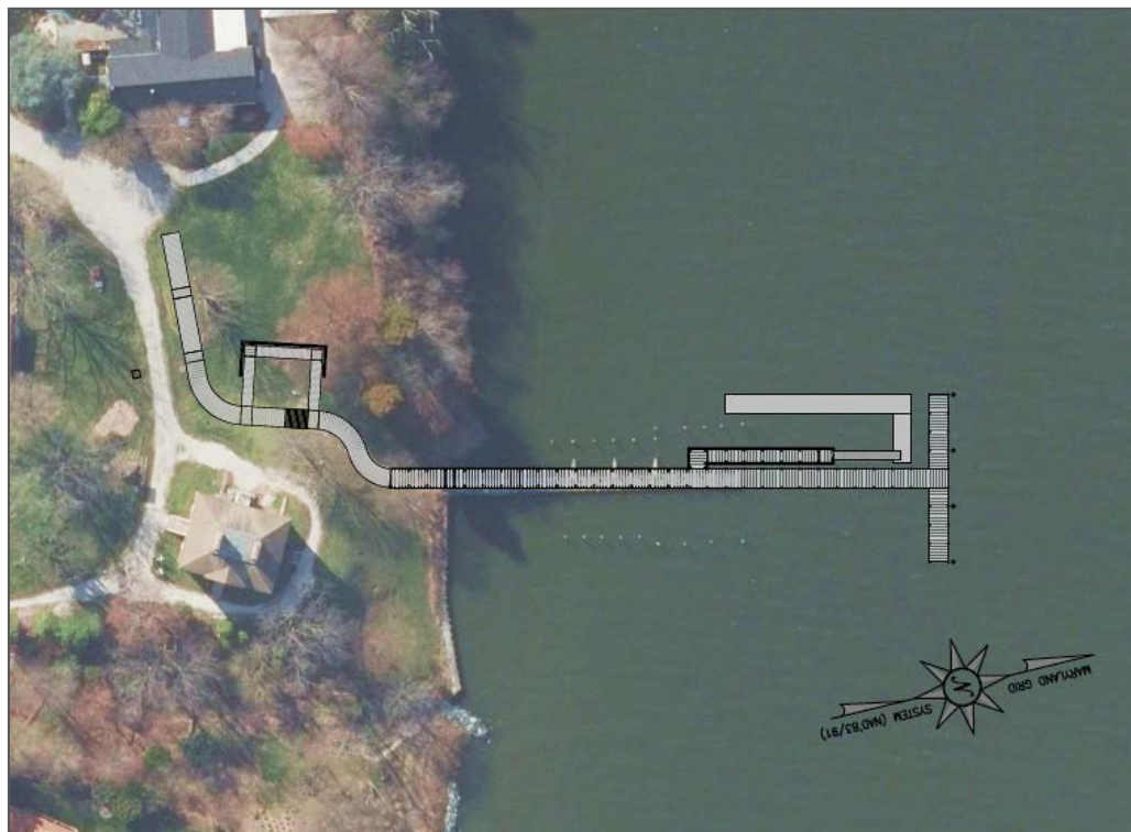
Figure 5 – ADA-Compliant Boardwalk and Main Pier
