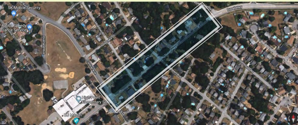
The walkzone for High Point Elementary School includes neighborhoods on both sides of Duvall Highway which is a two-lane roadway with shoulders and intermittent sidewalks. The walkzone could be expanded by installing sidewalks on the north side of Duvall Highway from Central Avenue to the existing sidewalk west of Pine Haven Drive. East of Pine Haven Drive, sidewalks on Duvall Highway connect to existing sidewalks along Queens Park Road
