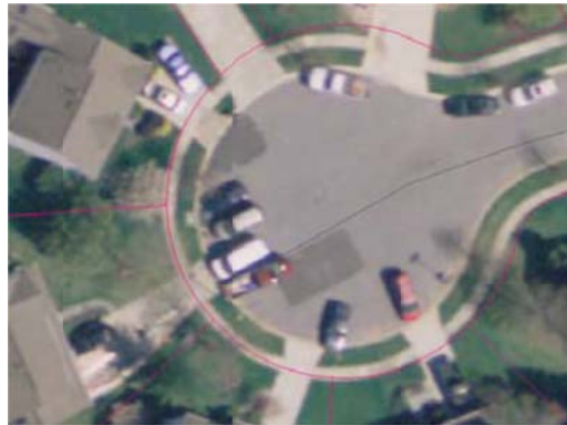
Figure 2 – Parking prevents plowing around the cul-de-sac
